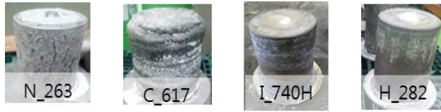
Fig. 1 Photograph of manufactured ingots by using the VIM+ESR process for superalloy
