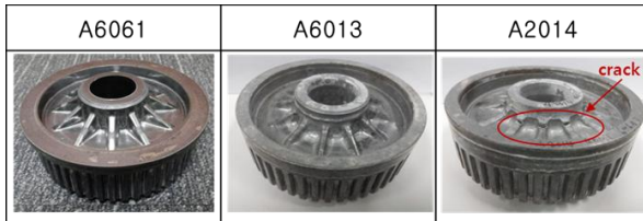
Fig. 1 A results of the formed rib and spline using A6061, A6013, A2014
